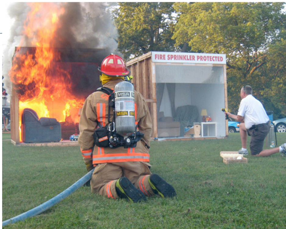
Reporting the temperature change as the fire grows into flashover on the unprotected side.
